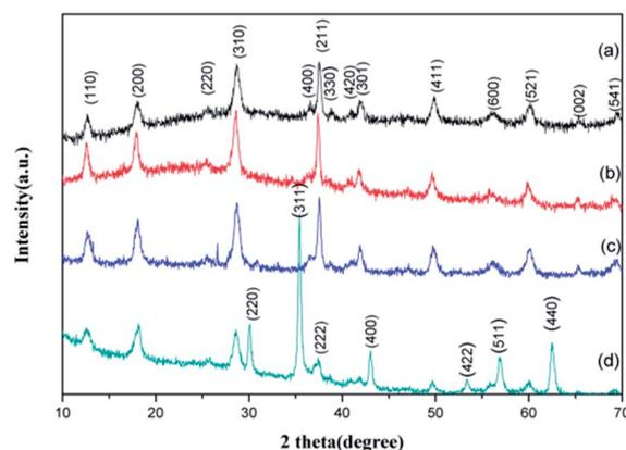
Fig. 3 X-ray diffraction patterns of (a) MnO<sub>2</sub>, (b) MnO<sub>2</sub>/PPy, (c) GO/MnO<sub>2</sub>, (d) GMFP.
