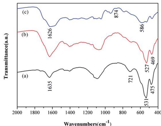
Fig. 4 FT-IR spectra of (a) MnO<sub>2</sub>, (b) MnO<sub>2</sub>/PPy, (c) GMFP nanocomposites.
