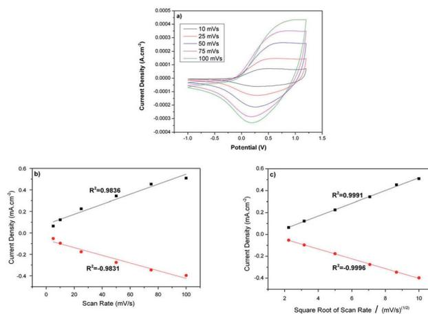
Fig. 3 (a) Cyclic voltammogram of PEDOT nanofibers in 0.1 M NBu<sub>4</sub>PF<sub>6</sub>/ACN at various scan rates, and plots of the anodic and cathodic peak current densities vs. (b) the scan rate, (c) the square root of the scan rate.
