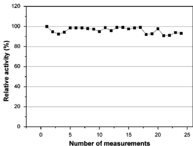
Fig. 8 Operational stability of the PEDOT-NFs/GOx-3 biosensor.
