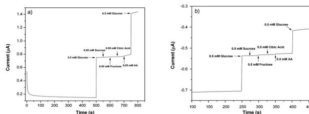
Fig. 9 Amperometric responses of (a) the PEDOT-NFs/GOx-3 (at 0.6 V) and (b) PEDOT-NFs/GOx-2 (at  $-0.6$  V) nanofiber biosensors versus sucrose, fructose, citric acid and AA (0.1 M PBS, pH 6.5, at 25 °C).
