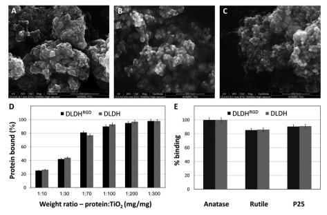
Fig. 2 Structure of  $TiO_2$  NPs forms and their binding to DLDH and DLDH<sup>RGD</sup>. ESEM micrographs of (A) A-NPs (B) rutile NPs and (C) P25-NPs. (D) Comparative binding of DLDH (gray) and DLDH<sup>RGD</sup> (black) to different  $TiO_2$  NPs preparations. (E) Binding curve of DLDH (gray) and DLDH<sup>RGD</sup> (black) at a 1:100 protein to  $TiO_2$  weight ratio. Experiments were repeated three times in triplicates. Average  $\pm$  stdev values are shown.
