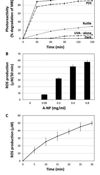
Fig. 1 TiO<sub>2</sub> nanoparticles photocatalytic activity. (A) Photodegradation of MB upon UVA illumination by the different preparations of TiO2. (B) ROS production by different amounts of A-NPs after 30 min of UVA illumination. (C) ROS production by a constant amount of A-NPs (0.4 mg ml<sup>-1</sup>) at different time intervals. Experiments were repeated three times in triplicates.
