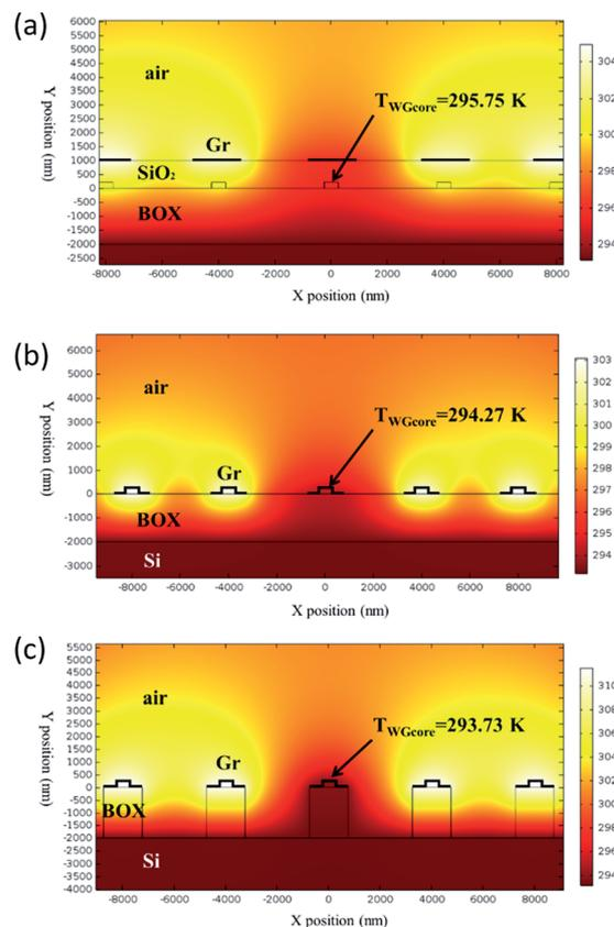
Fig. 11 Thermal field distributions of conventional structure with 1 μm-thick SiO<sub>2</sub> top cladding (a), graphene contact-heating structure without air trench (b) and with air trench (c).
