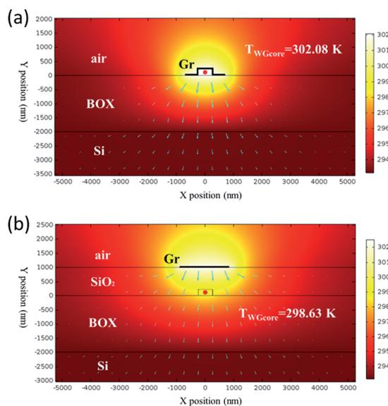
Fig. 4 Simulated thermal field distribution of the proposed structure with graphene contact heating (a) and the conventional structure with 1  $\mu\text{m}$ -thick top  $\text{SiO}_2$  cladding layer (b). Blue arrows shows the directions of heat flux.
