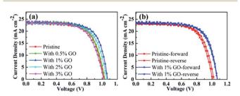
Fig. 1 (a) J-V curves of the fabricated champion PSCs with different amount of GO in the perovskite precursor solution; (b) the forward and reverse scans for the champion pristine PSC without GO and that with 1 vol% of GO.
