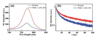
Fig. 5 (a) Steady-state photoluminescence (PL) and (b) time-resolved photoluminescence (TRPL) spectra of glass/MAPbl<sub>3</sub>/spiro-OMeTAD without or with 1 vol% GO.
