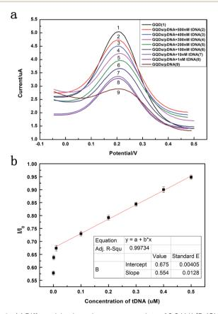
Fig. 6 (a) Differential pulse voltammograms plots of  $0.2 \, M \, K_3 [Fe(CN)_6]$  at pDNA (500 nM) immobilized GQDs modified GCE in 1.0 M KCl and that after hybridization with different concentrations of HBV-DNA (tDNA). (b) The plot of the peak current against the concentration of HBV-DNA.
