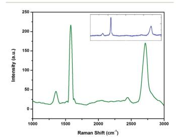
Fig. 1 Raman spectra of graphene and Talga expanded micro graphite (inset) showing D, G, and 2D peaks.
