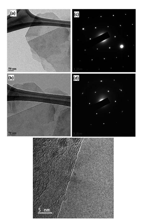
Fig. 2 TEM images [(a) and (b)] showing few layers of graphene and their corresponding diffraction patterns [c θ d] showing six-membered rings. (e) HRTEM images showing few layers of graphene.
