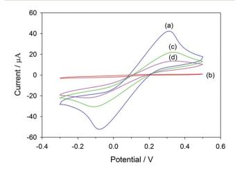
Fig. 1 Cyclic voltammograms of 5 mM  $\rm K_3[Fe(CN)_6]/K_4[Fe(CN)_6]$  in 100 mM KCl at (a) graphene/PEDOT:PSS/SPCE, (b) MIP electrode before template removal, (c) MIP electrode after template removal and (d) MIP electrode after target rebinding.
