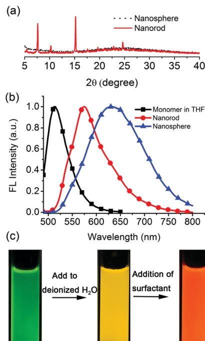
**Fig. 2** (a) The XRD patterns of the nanospheres and nanorods. (b) The emission spectra of the  $\text{BF}_2\text{bcz}$  monomer in THF, aqueous dispersions of the nanospheres and the nanorods. (c) The fluorescence images of the  $\text{BF}_2\text{bcz}$  monomer in THF (left), aqueous dispersions of nanospheres (middle) and nanorods (right) under illumination with a UV lamp.
