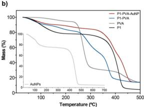
Fig. 2 (a) FT-IR spectra and (b) TGA profiles of the hydrogels and their components
