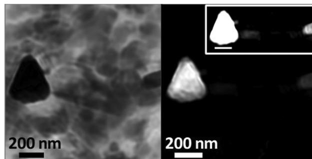
**Fig. 8** Ptychography image (710 eV; left) and iron contrast map (right) of iron deposit 2 located in the amyloid plaque core of Fig. 5(a–e). High contrast iron map (right; inset) shows additional iron detail in this region.
