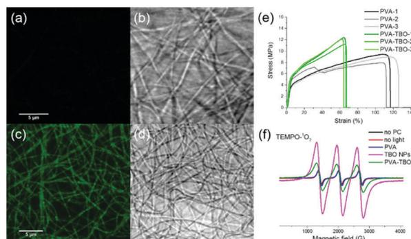
**Fig. 2** CLSM images of PVA (a and b) and PVA-TBO (c and d) nanofibrous membranes in the fluorescence mode (a and c) and transmission mode (b and d); (e) stress-strain curves of PVA and PVA-TBO membranes from 3 measurements; and (f) EPR spectra of TEMPO-<sup>1</sup>O<sub>2</sub> adducts from PVA, TBO NPs and PVA-TBO without and with light irradiation.
