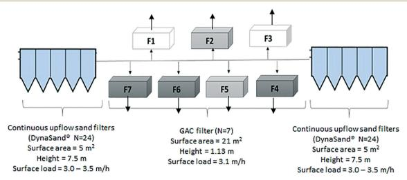
Fig. 1 Schematic of continuous-upflow sand filters and parallel downstream GAC filters in this study. Dark grey boxes (F4, F6, and F7) are modified GAC filters, light grey boxes (Rf2 and Rf5) are reference filters. Additional filters exist (F1 and F3), but were not studied in this experiment.
