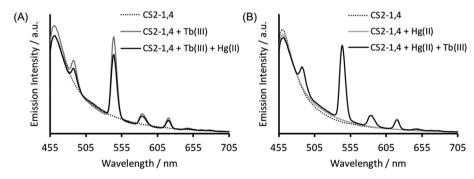
Fig. 3 Steady state luminescence spectra of 30  $\mu$ M CS2-1,4 monomer (dashed line) in the presence of 10  $\mu$ M TbCl<sub>3</sub> (grey line panel A), 10  $\mu$ M HgCl<sub>2</sub> (grey line panel B) or both 10  $\mu$ M TbCl<sub>3</sub> and 10  $\mu$ M HgCl<sub>2</sub> (black line) in 5 mM HEPES buffer pH 6.8 on order of addition of (A) TbCl<sub>3</sub> or (B) HgCl<sub>2</sub>, first.  $\lambda_{exc}$  = 280 nm.
