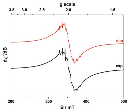
**Fig. 9** X-band EPR spectrum of **4** recorded in toluene solution at 293 K (experimental conditions: frequency, 9.8717 GHz; power, 0.63 mW; modulation, 0.3 mT). Experimental data are represented by the black line; simulation is depicted by the red trace.
