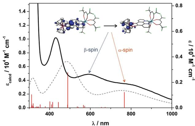
**Fig. 11** Overlay of the experimental (solid line) and calculated (dashed line) electronic absorption spectra for **3**. The vertical bars show the individual calculated transitions. Inset orbitals depict the HOMO–1 → LUMO transition that constitutes the two lowest energy bands designated the  $\alpha$ -spin and  $\beta$ -spin excitations, respectively.
