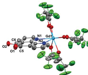
Fig. 2 Molecular structure of **2a**. Hydrogen atoms and  $\text{Et}_2\text{O}$  of crystallisation omitted for clarity. Thermal ellipsoids drawn at 50% probability. Selected distances (Å): Gd1–N1 2.585(8), Gd1–N2 2.555(9), C5–C6 1.54(6), C6–O2 1.23(2), C5–O1 1.24(2).
