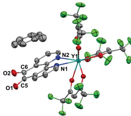
Fig. 1 Molecular structure of **1b**. Hydrogen atoms omitted for clarity. Thermal ellipsoids drawn at 50% probability. Selected distances (Å): Y1–N1 2.501(3), Y1–N2 2.552(3), C5–C6 1.524(6), C6–O2 1.216(5), C5–O1 1.213(5).
