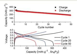
Fig. 5 Galvanostatic cycling of tin phosphide vs. Prussian Blue using electrolyte of 1 M NaPF<sub>6</sub> dissolved in EC: DEC (1:1) with 10 vol% FEC. The cell utilized an oversized cathode and capacity is based on the active material in the anode
