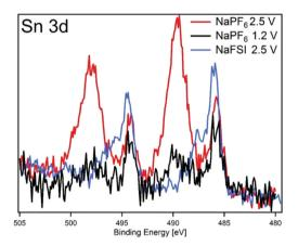
Fig. 7 HAXPES spectra of Sn 3d orbital using photon energy of 2005 eV for: NaPF $_6$  charged to 1.2 V (black) and 2.5 V (red) and NaFSI charged to 2.5 V (note NaFSI sample electrolyte contained 5 vol% FEC).
