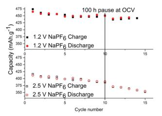
Fig. 3 Discharge and charge capacities in tin-phosphide half-cells using NaPF $_6$  before and after 100 h pause/relaxation. Top figure shows the results for the cell with 1.2 V high cut-off potential, and the bottom figure displays for the cell with 2.5 V high cut-off potential.
