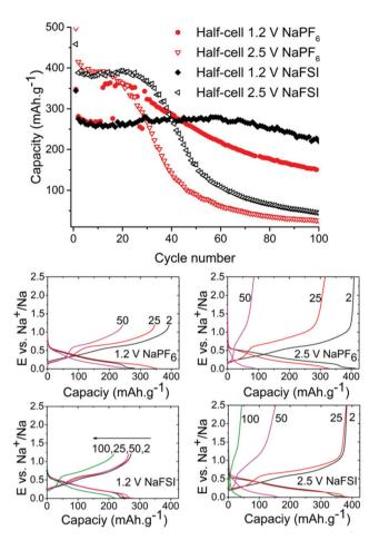
**Fig. 2** Discharge capacity from galvanostatic cycling of tin phosphide at 50 mA  $\rm g^{-1}$  in half cells with NaFSI (black) & NaPF<sub>6</sub> (red) with upper cut-off potential set to 1.2 V and 2.5 V (top). Voltage profiles for same cells at selected cycles (bottom).
