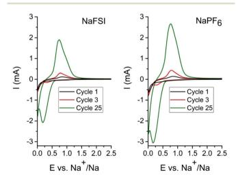
Fig. 1 Cyclic voltammogram of  $Sn_4P_3$  vs. sodium metal using electrolytes of 1 M NaFSI (left) or  $NaPF_6$  (right) dissolved in EC:DEC (1:1) and 10 vol% FEC additive. Scan was performed between 0.01 V–2.5 V at 1 mV s<sup>-1</sup> scan rate.
