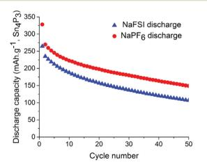
Fig. 4 Discharge capacity for symmetrical-cells with NaPF $_6$  salt (red) and NaFSI salt (blue) over 50 galvanostatic cycles. Electrodes were cycled between -1.25 V and 1.25 V in pouch cells.
