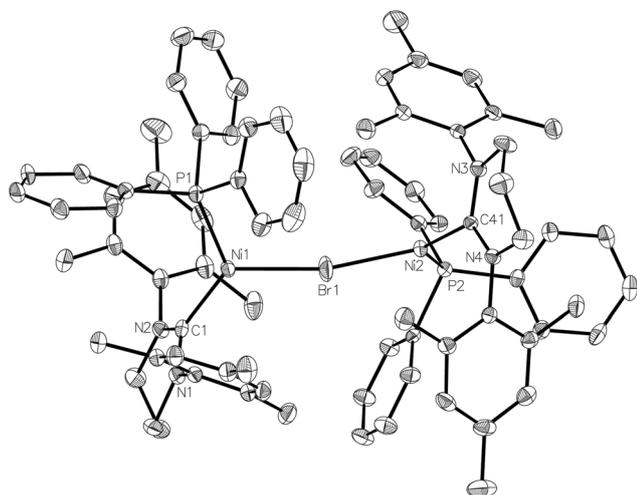
**Fig. 3** Molecular structure of the cation in **3**. Ellipsoids are shown at the 30% probability level. Hydrogen atoms have been omitted for clarity. Selected bond lengths (Å) and angles (°): Ni(1)–C(1) 1.937(4), Ni(1)–P(1) 2.2172(12), Ni(1)–Br(1) 2.3803(6), Ni(2)–C(41) 1.935(4), Ni(2)–P(2) 2.2186(11), Ni(2)–Br(1) 2.3688(6), C(1)–Ni(1)–P(1) 124.15(11), C(1)–Ni(1)–Br(1) 122.16(11), P(1)–Ni(1)–Br(1) 113.68(4), Ni(1)–Br(1)–Ni(2) 167.64(3).
