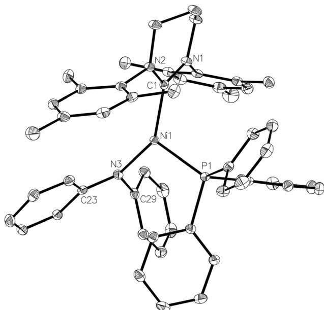
**Fig. 8** Molecular structure of **8**. Ellipsoids are shown at 30% probability. Hydrogen atoms and the minor disordered component of C3 have been omitted for clarity. Selected bond lengths (Å) and angles (°): Ni(1)–C(1) 1.9612(14), Ni(1)–P(1) 2.2337(4), Ni(1)–N(3) 1.9350(12), C(1)–Ni(1)–P(1) 109.25(4), C(1)–Ni(1)–N(3) 142.47(5), P(1)–Ni(1)–N(3) 108.13(4).
