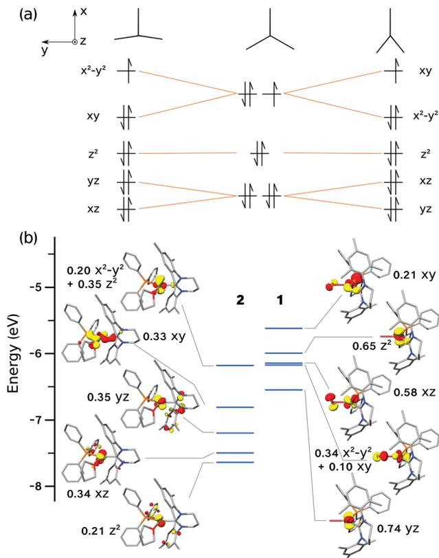
**Fig. 10** (a) Schematic molecular orbitals diagrams expected for three-coordinate  $d^9$  complexes, left to right: T-shaped, ideal  $D_{3h}$ , Y-shape; a larger ligand field splitting would lead to crossings of MO energy levels. (b) Quantitative MO diagrams for complexes **1** (right) and **2** (left) based on energies and characters of spin-up orbitals.
