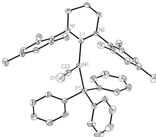
**Fig. 5** Molecular structure of the cation in **5**. Ellipsoids are shown at the 30% probability level. Hydrogen atoms have been omitted for clarity. Selected bond lengths (Å) and angles (°): Ni(1)–C(1) 1.943(3), Ni(1)–C(23) 1.787(3), Ni(1)–P(1) 2.2374(8), C(23)–O(1) 1.132(4), C(1)–Ni(1)–P(1) 151.93(9), C(1)–Ni(1)–C(23) 106.24(13), P(1)–Ni(1)–C(23) 101.76(11), O(1)–C(23)–Ni(1) 178.0(3).
