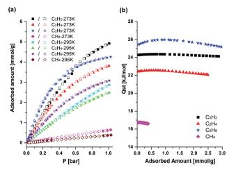
Fig. 3 (a) The adsorption isotherms of HOF-BTB for C<sub>2</sub>H<sub>2</sub>, C<sub>2</sub>H<sub>4</sub>, C<sub>2</sub>H<sub>6</sub> and CH<sub>4</sub> at 273 K and 295 K, respectively, and (b) loading dependent isosteric heat  $(Q_{st})$  of adsorption. The  $Q_{st}$  values were calculated based on adsorption isotherms at 273 K and 295 K by using the Virial method.
