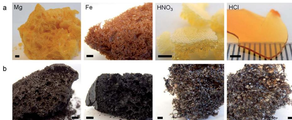
Fig. 2 Images of  $\text{Mg}(\text{NO}_3)_2$ /gelatin,  $\text{Fe}(\text{NO}_3)_3$ /gelatin,  $\text{HNO}_3$ /gelatin, and HCl/gelatin foams after (a) drying and (b) carbonization at 800 °C (scale bars 2 mm).
