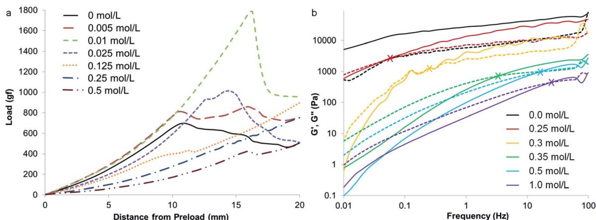
Fig. 3 (a) Load vs. distance plot showing the breaking point for gelatin gels at 10% w/v with different concentrations of iron nitrate. (b) Plots of storage modulus ( $G'$ , solid lines) and loss modulus ( $G''$ , dashed lines) against frequency for gelatin at 20% w/v with different concentrations of iron nitrate.
