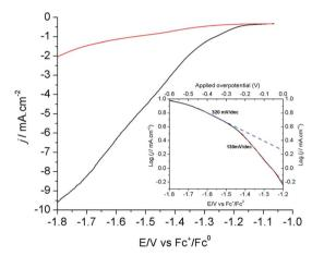
Fig. 3 LSVs of the modified Cu electrode (80 s electrodeposition) in N<sub>2</sub>- (red) and CO<sub>2</sub>-saturated (black) [EMIM](BF<sub>4</sub>)/H<sub>2</sub>O (92/8 v/v). Inset: Tafel plot for the electrode in CO<sub>2</sub>-saturated [EMIM](BF<sub>4</sub>)/H<sub>2</sub>O (92/8 v/v).
