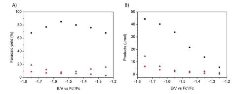
Fig. 2  $CO_2$  reduction products recorded on a modified Cu electrode (80 s electrodeposition) as a function of applied potential: faradic yields (A) and absolute amounts (B) of formate (black squares), CO (red circles) and H<sub>2</sub> (blue triangles) during 30 minutes electrolysis in  $CO_2$ -saturated [EMIM](BF<sub>4</sub>)/H<sub>2</sub>O (92/8 v/v).
