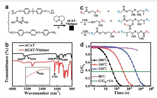
Fig. 1 Polymer synthesis and characterization. (a) Synthesis of ACAT–vitrimer. (b) FTIR spectra of ACAT and ACAT–vitrimer. (c) An illustration of reversible transesterification. (d) Stress relaxation experiments of ACAT–vitrimer at different temperatures.
