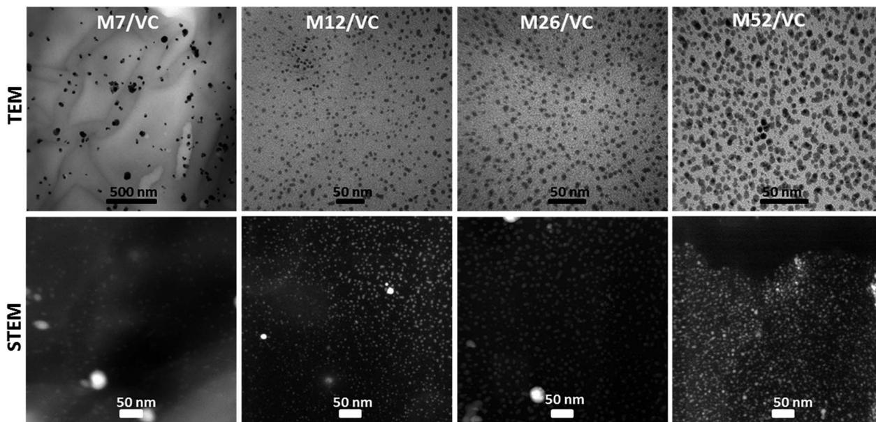
Fig. 3 TEM (top row) and STEM-HAADF (bottom row) images of chitosan medium and ascorbic acid-based films MAg/VC with increasing silver content. A uniform distribution of nanoparticles across the film is visible. The presence of large agglomerates is excluded even with the highest silver loading.
