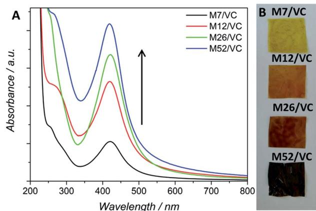
Fig. 1 (A) UV-Vis absorption spectra for chitosan medium  $M_w$  and ascorbic acid (M/VC) based AgNPs (for 7, 12, 26 and 52 mM silver precursor). Surface plasmon resonance band (SPR) at  $\sim 420$  nm appears due to the common excitation of the nanoparticle free electrons. Black arrow depicts the increasing concentration of AgNPs. (B) Photographs of chitosan–silver films with different AgNP loadings (7, 12, 26 and 52 mM  $\text{Ag}^+$  initial concentration, respectively).
