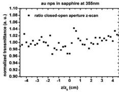
Fig. 4 Nonlinear refraction for the isotropic Au NPs in  $\alpha$ -Al<sub>2</sub>O<sub>3</sub> at 532 nm and 355 nm. For the first wavelength, the nonlinear optical refraction is positive, whereas it is null for the second wavelength. 41
