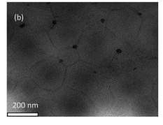
Fig. 15 The TEM images of the thin films prepared from the dispersions produced by the dispersion copolymerization of BA and HFBA in the presence of Pol-A in the methanol-water mixture with the following composition: 80:20 (a) and 70:30 vol% (b), and after the dialysis
