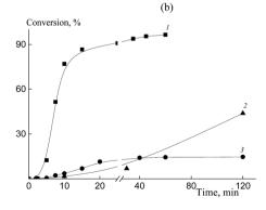
Fig. 1 The time dependence of the conversion in the copolymerization of acrylic acid and HFBA (a), acrylic acid and OFPA (b) in DMF at 80 °C in the presence of BTC and AIBN (1  $\times$  10<sup>-3</sup> mol L<sup>-1</sup>). (a) [BTC] = 0 (1, 3) and 6  $\times$  10<sup>-3</sup> mol L<sup>-1</sup> (2), HFPA in the feed: 10 (1, 2) and 50 mol% (3); (b) [BTC] = 6  $\times$  10<sup>-3</sup> mol L<sup>-1</sup>, OFPA in the feed: 10 (1), 20 (2) and 30 mol% (3).
