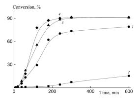
Fig. 13 Dependence of monomer conversion on the reaction time for the dispersion copolymerization of BA and HFBA in the methanolwater mixture at 65 °C in the presence of BTC (1) and Pol-A (2–4), [BTC] = [Pol-A] =  $2.2 \times 10^{-3}$  mol L<sup>-1</sup>, [AIBN] =  $1.1 \times 10^{-3}$  mol L<sup>-1</sup>, 10 mol% of HFBA. Volume ratio (%) of methanol : water = 90:10 (2), 80:20 (3), and 70:30 (1, 4).
