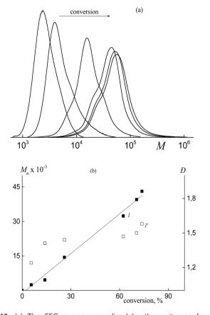
Fig. 12 (a) The SEC curves normalized by the unit area for the copolymers of butyl acrylate and HFBA synthesized in the presence of BTC by the dispersion polymerization. HFBA, 10 mol% in monomer feed, methanol : water = 70 : 30 vol%, monomers : media = 1 : 7 v/v, [BTC] =  $2.2 \times 10^{-3}$  mol L<sup>-1</sup>, [AIBN] =  $1.1 \times 10^{-3}$  mol L<sup>-1</sup>. (b) Dependences of  $M_{\rm n}$  (1) and D (1') on conversion for the synthesized copolymers.
