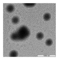
Fig. 11 The TEM images of the films after emulsion copolymerization of BA and OFPA in the presence of Cop-O2 and drying of the asformed dispersions.
