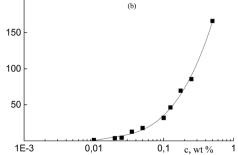
Fig. 7 (a) Surface tension isotherms for aqueous solutions containing 0.1 M NaCl of polymer Pol-A (1) and copolymers Cop-H2 (2), Cop-O2 (3) and Cop-O10 (4) at pH 5.4 and  $T=25\,^{\circ}\mathrm{C}$  on the water–air interface. (b) Dependence of number-average diameters of the particles  $D_{\mathrm{n}}$  in aqueous solution containing 0.1 M NaCl of copolymer Cop-O2 on its concentration at pH 5.4 and  $T=25\,^{\circ}\mathrm{C}$ .
