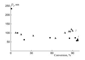
Fig. 9 Dependences of number-average diameter  $D_n$  of the particles on monomer conversion in the emulsion polymerization initiated by PSK at 70 °C. Monomers: water = 1:4 v/v, [BA]/[OFPA] = 80/20 mol mol<sup>-1</sup>, Cop-O2 (1), Cop-O10 (2).
