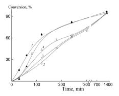
Fig. 4 The time dependence of the conversion for the copolymerization of butyl acrylate and HFBA in DMF initiated by AIBN (5  $\times$  10 $^{-4}$  mol L $^{-1}$ ) in the presence of the RAFT agent (3  $\times$  10 $^{-3}$  mol L $^{-1}$ ). The RAFT agent: BTC (1), Pol-A (2–4) and Cop-H5 (5). Butyl acrylate : HFBA = 90 : 10 (1, 2), 85 : 15 (3), 80 : 20 (4, 5). Total monomer concentration is 2 mol L $^{-1}$ .
