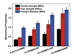
Fig. 7 Comparison of tensile and tear strength of pure H-t-PDMS and its nanocomposites filled with 0.5 wt% various carbon nanofillers including CNTs, f-CNTs and GONRs.
