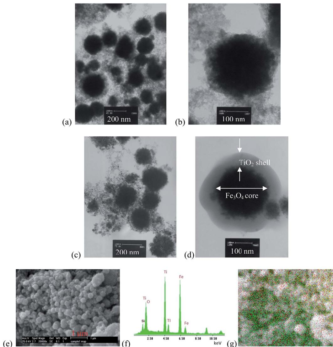
Fig. 5 TEM micrographs of (a)  $\text{Fe}_3\text{O}_4$  nanoparticles, (b) single core of  $\text{Fe}_3\text{O}_4$  nanoparticles (c)  $\text{Fe}_3\text{O}_4@TiO_2$  nanoparticles, (d) and single core-shell of  $\text{Fe}_3\text{O}_4@TiO_2$  (e) SEM, (f) EDX spectra of  $\text{Fe}_3\text{O}_4@TiO_2$  core-shell and (g) EDX point image taken from core-shell  $\text{Fe}_3\text{O}_4@TiO_2$  nanoparticle marked in the SEM images.
