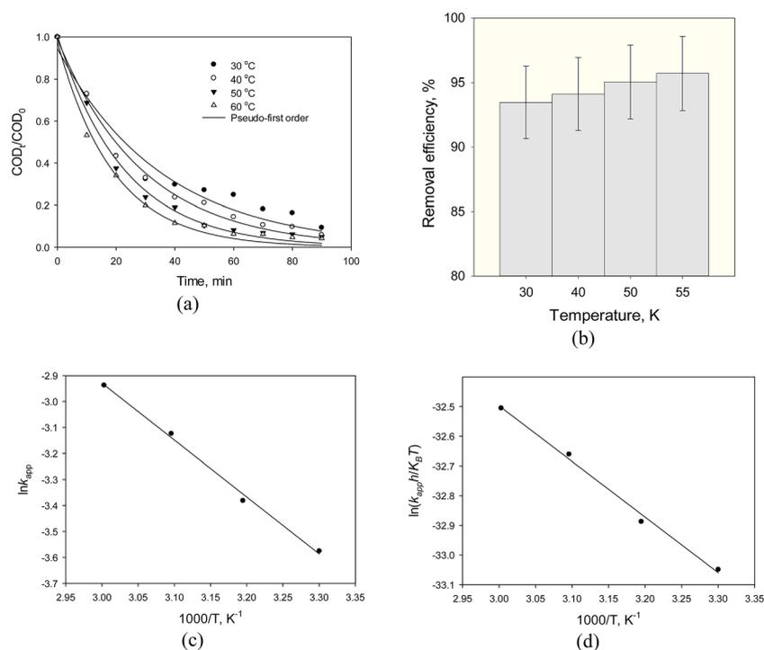
Fig. 11 (a) Kinetic curves, (b) removal efficiency, (c) the Arrhenius plot and (d) the Eyring plot of SMW with  $\text{Fe}_3\text{O}_4@\text{TiO}_2$  (FT1) at different temperature (photocatalyst dose  $1 \text{ g L}^{-1}$ , pH = 3,  $920 \text{ mg L}^{-1}$  initial COD, and 90 min reaction time).
