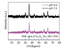
Fig. 16 XRD patterns of the magnetic PPy-GO after use.
