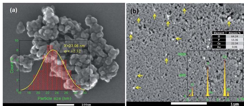
**Fig. 5** Typical SEM images of (a) 600 °C air annealed HAp, and (b) 0.055 wt% Au–HAp nanocomposites. The inset of (a) presents size distribution histogram of the pristine HAp nanoparticles. A typical EDS spectrum of the Au-loaded sample is presented as inset of (b). Presence of Au nanoparticles at the surface of HAp nanoparticles (indicated by arrows) can be noticed from their brighter contrasts.
