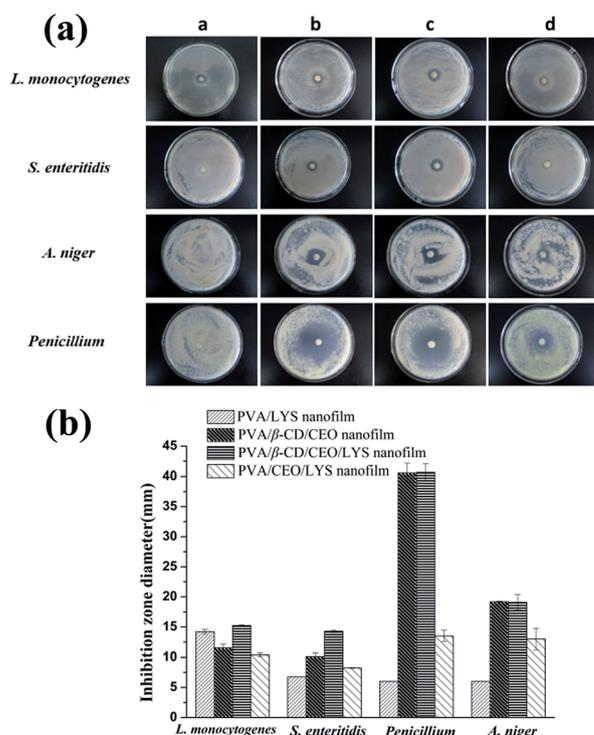
Fig. 8 Inhibition zones (a) and the corresponding diameter (b) of different electrospun nanofilms against *L. monocytogenes*, *S. enteritidis*, *A. niger* and *Penicillium*. (a: PVA/LYS nanofilm; b: PVA/ $\beta$ -CD/CEO nanofilm; c: PVA/ $\beta$ -CD/CEO/LYS nanofilm; and d: PVA/CEO/LYS nanofilm).
