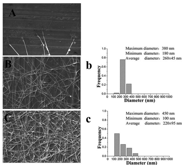
**Fig. 3** SEM images of the electrospun nanofilm with different  $\beta$ -CD concentrations (A: 1%  $\beta$ -CD; B: 2%  $\beta$ -CD; and C: 3%  $\beta$ -CD) and fiber diameter distribution of the electrospun nanofilm (b: PVA/CEO/LYS/2%  $\beta$ -CD and c: PVA/CEO/LYS/3%  $\beta$ -CD).
