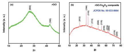
Fig. 1 PXRD spectra of (a) rGO and (b) rGO-Fe<sub>2</sub>O<sub>3</sub> composite.
