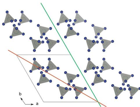
Fig. 1 Schematic of identifying growth planes in ZIF-8. The organic linkers are suppressed and lighting is turned out in VESTA<sup>28</sup> for clarity. Orange: the (110) plane is not allowed, as it cannot be drawn without dissecting linker units. Green: the (100) plane is allowed as it can be drawn without dissecting linker unit.
