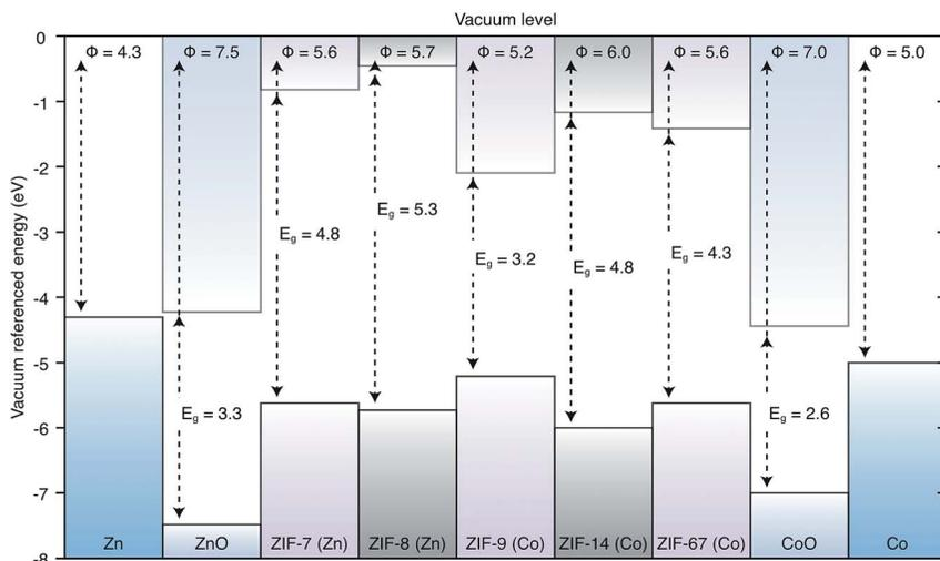
Fig. 2 Band alignment of ZIFs. IPs ( $\phi$ ) and band gaps ( $E_g$ ) are given for each framework and for the metal oxides in units of eV. The workfunctions of the contact metals are given at either end. The label of each framework indicates the metal linker node upon which it is based.
