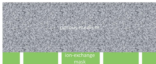
Fig. 1 Sketch of a nano-porous layer sandwiched with a perforated ion-exchange mask (not to scale).
