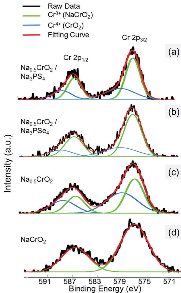
Fig. 7 XPS spectra of Cr 2p from the surfaces of (a) mixture of  $\text{Na}_{0.5}\text{CrO}_2$  and  $\text{Na}_3\text{PS}_4$  at RT (25 °C), (b) mixture of  $\text{Na}_{0.5}\text{CrO}_2$  and  $\text{Na}_3\text{PSe}_4$  at RT (25 °C), (c)  $\text{Na}_{0.5}\text{CrO}_2$ , and (d)  $\text{NaCrO}_2$ .
