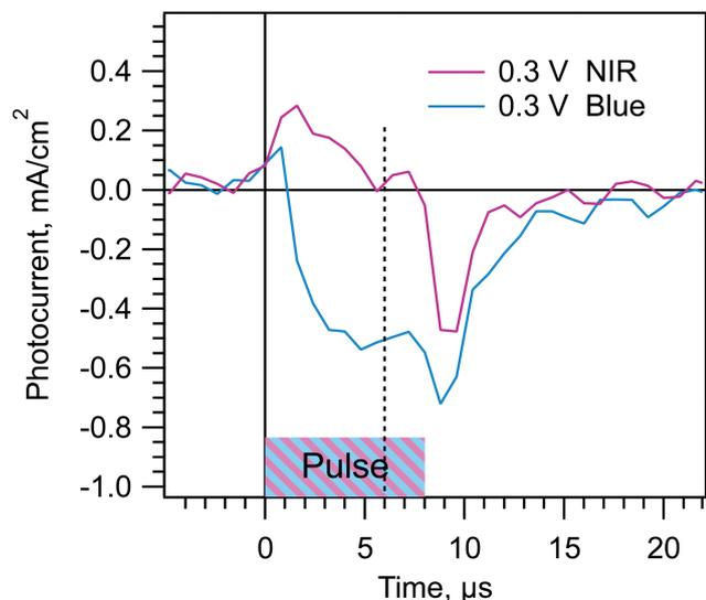
Fig. 5 Effect of blue vs. NIR (735 nm) pulses at  $V_{\text{d}}$  and  $t_{\text{d}}$  where the photocurrents from regions I and III vs. region II are balanced for the NIR pulse. The peaks at 1  $\mu\text{s}$  and 9  $\mu\text{s}$  are from the switching of the LED. Data from a m-TiO<sub>2</sub>/MAPI cell with  $t_{\text{d}} = 2$  ms and  $V_{\text{d}} = 0.3$  V.
