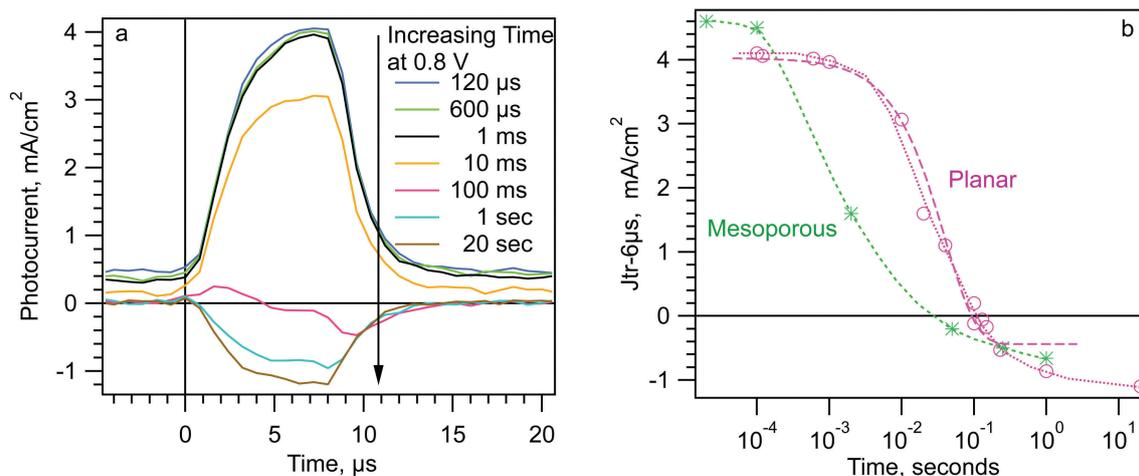
Fig. 3 (a) Photocurrent transients from the SDP experiment for a dwell voltage of 0.8 V and various dwell times. (b)  $J_{tr}$ -6 $\mu$ s vs. dwell time at dwell voltage 0.8 V for the planar and mesoporous cells used in Fig. 1 and 2.
