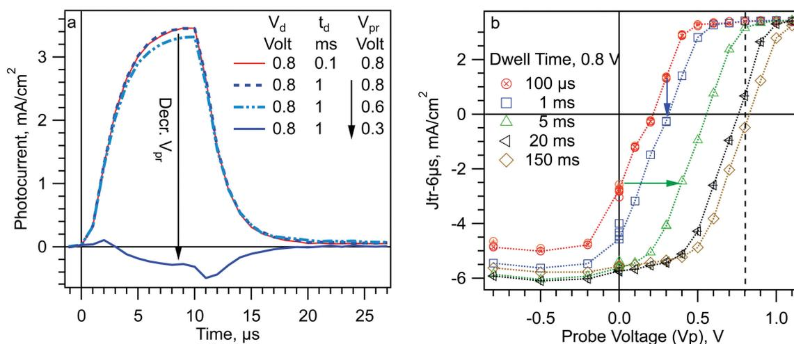
Fig. 4 Results of SDSP experiments on a planar MAPI cell. (a) Example photocurrent transients for a dwell voltage ( $V_d$ ) of 0.8 V. (b)  $J_{\text{tr}-6\mu\text{s}}$  vs.  $V_{\text{pr}}$  and  $t_d$ , from SDSP experiments using a dwell voltage of 0.8 V.
