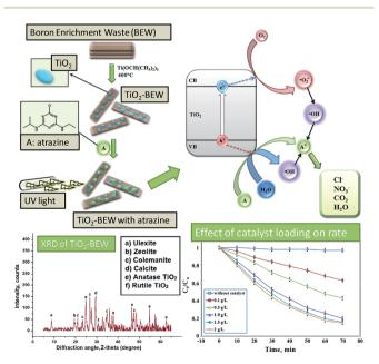
Fig. 8 TiO<sub>2</sub> photocatalyst supported on boron enriched waste and its use in atrazine photodegradation. Adapted from ref. 141. Copyright 2014, with permission from Elsevier.
