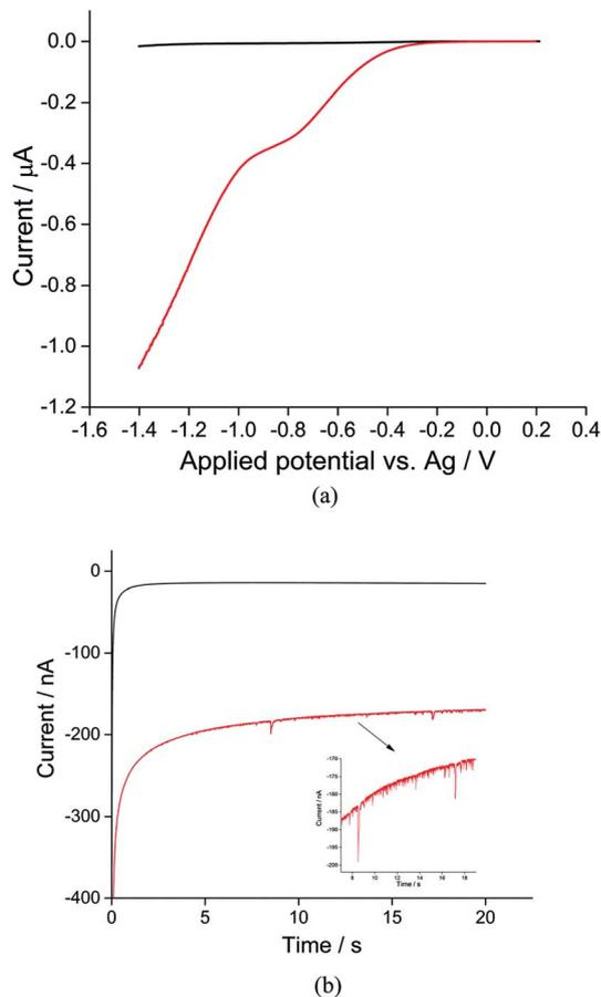
Fig. 1 (a) Linear sweep voltammograms and (b) chronoamperograms at  $-1.4$  V vs. silver pseudo-reference electrode of the toluene emulsion taken in the nitrogen-degassed (black) and oxygenated (red) states using a microwire electrode. If cyclic voltammetry is recorded in (a) the reverse scan is essentially superimposed on the forward scan.
