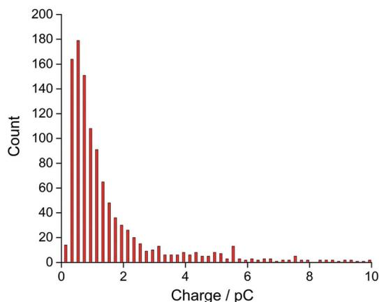
Fig. 3 Distribution of charge of the nano-impact spikes observed in toluene emulsion droplets at  $-1.4$  V vs. silver pseudo-reference electrode.
