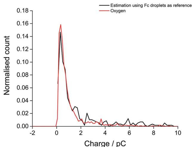
Fig. 5 The distribution of experimental charge obtained from oxygen reduction of individual toluene droplets (red) and the charge distribution from theoretical estimation (black) using eqn (2) ( $C_{\text{oxygen}} = 27$  mM).
