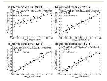
Fig. 4 Linear free energy scaling relationships amongst intermediates for the kinetic steps of olefin hydroformylation without consideration of different ligand size. The mathematical equations that define the linear scaling relationships are used to create the simulated reaction profile and, ultimately, the final volcano plot (vide infra).
