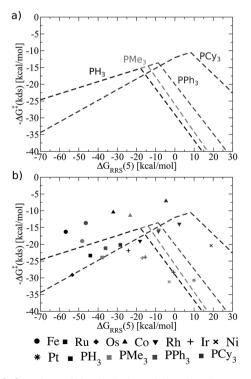
Fig. 8 (a) Overview of the hydroformylation kinetics separated by ligand type, as derived from the linear free energy scaling relationships that define the catalytic cycle depicted in Fig. 2. (b) Volcano plot illustrating the kinetic suitability of catalysts derived from (a)
