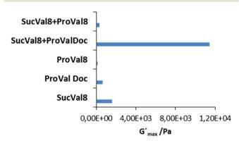
Fig. 3 Comparison of  $G'_{\mathrm{max}}$  of different gels. The plateau region of the graph was taken as the  $G'_{\text{max}}$  of each system (Fig. S9†).
