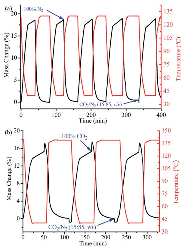
Fig. 4 Repeated adsorption–desorption kinetics for **1a** (a) between a 15 : 85 CO<sub>2</sub>/N<sub>2</sub> (v/v) flow at 313 K and a pure N<sub>2</sub> flow at 403 K and (b) between a 15 : 85 CO<sub>2</sub>/N<sub>2</sub> (v/v) flow at 313 K and a pure CO<sub>2</sub> flow at 413 K.
