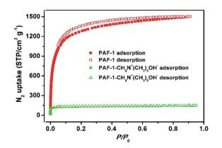
Fig. 1  $\rm N_2$  sorption isotherms of PAF-1 (red) and PAF-1-CH $_2$  -  $\rm N^+(CH_3)_3OH^-$  (green).
