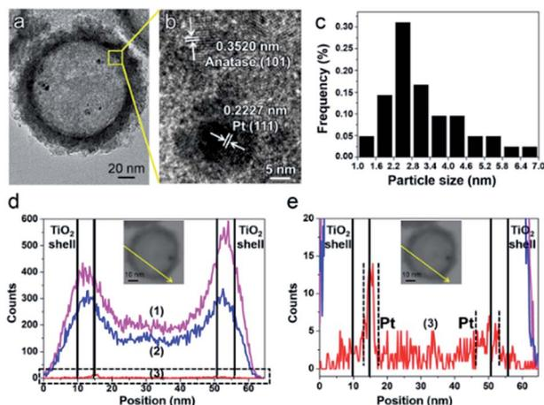
Fig. 3 The confirmation of PT-HS structures. (a) TEM image of a PT-HS. (b) HRTEM image of the area near the inner surface of the  $\text{TiO}_2$  shell. (c) The distribution of the particle size. (d) EDS line scan of a PT-HS. The part in the dotted pane is magnified in image (e). (e) The magnified patterns of the EDS line scan. Inset in image (d) and (e): the path of the EDS line scan. Curves (1), (2) and (3) in image (d) and (e) refer to the signals of Ti, O and Pt, respectively.
