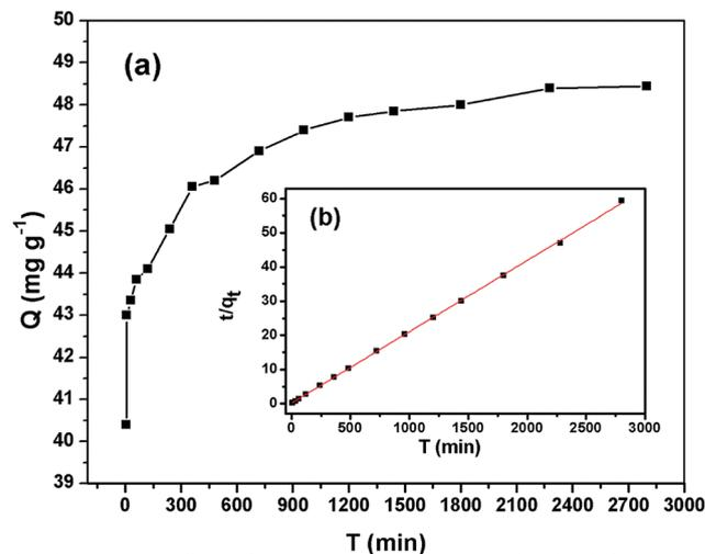
Fig. 6 Kinetics of Cr(vi) adsorption onto the  $\beta$ -CCWB450 at 298.15 K. (a) Cr(vi) sorption kinetics data, (b) pseudo-second-order model for Cr(vi) adsorption (initial Cr(vi) concentration 100  $\text{mg L}^{-1}$ ; pH = 2.0).
