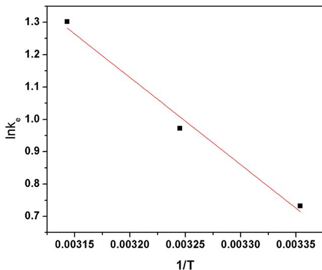
**Fig. 8** Plot of  $\ln k^0$  versus  $T^{-1}$  for estimation of thermodynamic parameters for the adsorption of Cr(vi) on  $\beta$ -CCWB450 (Cr(vi) solution volume: 50 mL; adsorbent dose: 0.1 g; initial Cr(vi) concentration: 20, 50, 100, 200, 300, 400, 500, 600, 800 mg L<sup>-1</sup>; contact time: 24 h; pH: 2.0).
