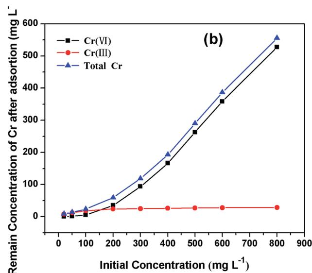
Fig. 11 (a) Time variation of Cr(III), Cr(vi) and total Cr concentration (initial Cr(vi) concentration: 100 mg L<sup>-1</sup>; Cr(vi) solution volume: 50 mL; adsorbent dose: 0.1 g; pH: 2.0), (b) initial concentration variation of Cr(III), Cr(vi) and total Cr concentration after adsorption (Cr(vi) solution volume: 50 mL; contact time: 24 h; adsorbent dose: 0.1 g; pH: 2.0).
