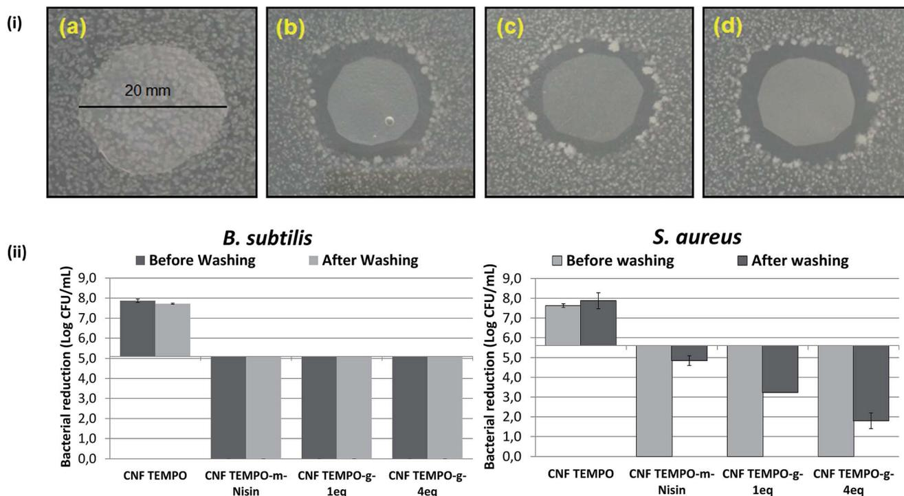
Fig. 7 (i) Qualitative analysis of grafting on antimicrobial activity of *B. subtilis*: (a) CNF Tempo (b) CNF Tempo-m-nisin (c) CNF Tempo-g-1-eq. (d) CNF Tempo-g-4eq., (ii) effect of nisin on antimicrobial activity of *Bacillus subtilis* and *Staphylococcus aureus* on CNF Tempo, CNF Tempo-m-nisin, CNF Tempo-g-1-eq., and CNF Tempo-g-4eq.
