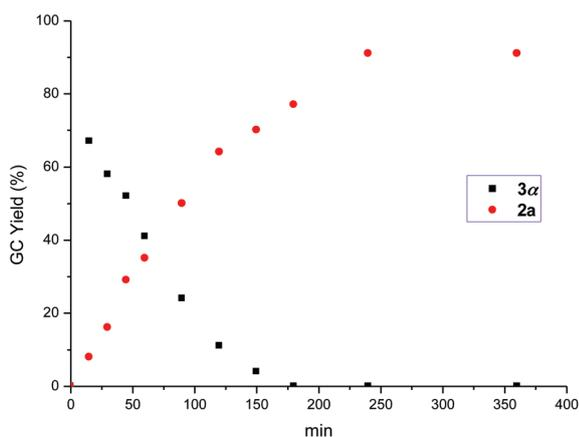
**Fig. 1** Profile of sequential hydroboration of 1-hexyne (**1a**) with 2 equiv. of HBpin catalyzed by 3 mol% **4b** and 6 mol% NaBHET<sub>3</sub> in THF at room temperature.
