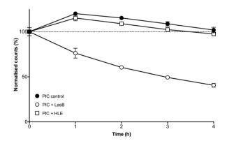
Fig. 4 Normalised detection counts (%) for P1<sub>SH</sub> PIC nanoparticles prepared at a 1:0.3 N: COOH ratio in the absence ( $\bullet$ ) and presence of LasB ( $\circ$ ) and HLE ( $\circ$ ). Data normalised to the initial counts for each of the individual experiments. n=3.
