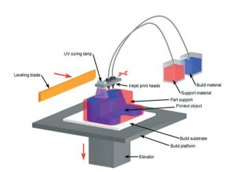
Fig. 5 Photopolymer based inkjet printer.<sup>20</sup> (Copyright 2008 Custom Part Net).
