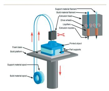
Fig. 17 Schematic illustration of FDM 3D printer. The feedstock filament of thermoplastic material is drawn from a spool into the FDM extrusion head, in which it is heated into a semiliquid state and then by drive wheels it is extruded out through nozzle on a built platform.<sup>20</sup> (Copyright 2008 Custom Part Net).
