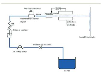
Fig. 2 Schematic illustration of DoD printing process.
