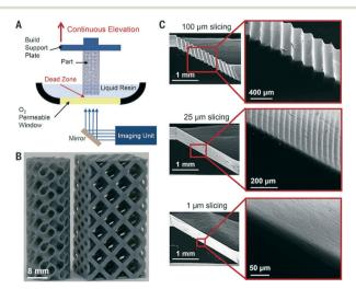
Fig. 13 (A) Schematic illustration of CLIP printer. (B-C) CLIP enables fast print speeds and layerless part construction.<sup>68</sup> (Copyright 2015 AAAS).
