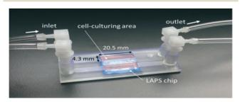
Fig. 10 LAPS chip with attached microfluidic channels.<sup>54</sup> (Copyright 2015 WILEY).
