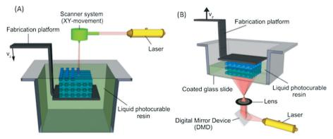
Fig. 7 Two SLA printing configurations. (A) Laser-scanning SL with the free surface/bath configuration. (B) DLP SLA with the constrained-surface/"bat" configuration. (Copyright 2015 Elsevier).
