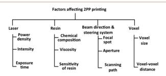
Fig. 15 Parameters affecting 2PP print process.
