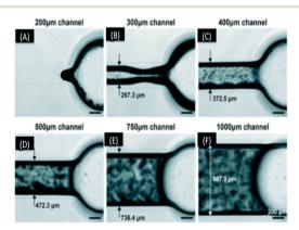
Fig. 11 (A–F) Micrographs of 500  $\mu$ m tall channels built in a range of widths. The actual width of each channels showed deviation of almost 30  $\mu$ m from design. The 300  $\mu$ m wide channel could only be partially cleared of resin, while the smaller channels did not clear at all and larger channels were fully cleared. <sup>60</sup> (Copyright 2015 RSC).
