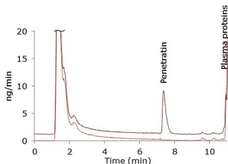
**Fig. 3** Mass flow chromatogram from LC-ICP-MS/MS. 50  $\mu\text{M}$  Pen spiked in 50% plasma prior to sample pre-treatment and 50% blank plasma. Dark red: Pen in plasma, light red: blank plasma, offset by  $-1.2$   $\text{ng min}^{-1}$ .
