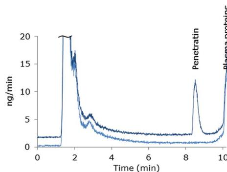
Fig. 1 Mass flow chromatograms from LC-MD-ICP-DRC-MS analysis of 50% plasma samples. Light blue: blank plasma, offset by  $-1.2 \text{ ng min}^{-1}$ . Dark blue: 50  $\mu\text{M}$  Pen spiked in 50% plasma prior to sample pre-treatment.
