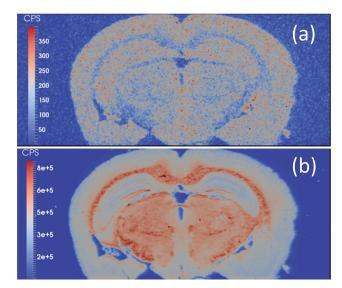
Fig. 3 (a)  $^{80}$ Se  $\rightarrow$   $^{80}$ Se $^{16}$ O image and (b)  $^{31}$ P  $\rightarrow$   $^{31}$ P $^{16}$ O image of a mouse brain obtained with LA-ICP-QQQ and an O2/H2 tune.
