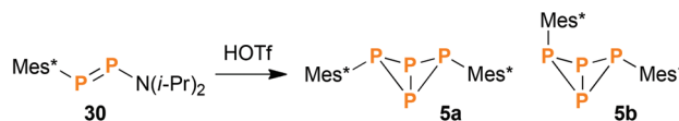
Scheme 3 Reaction of diphosphene 30 with HOTf, yielding bicyclic phosphanes 5a and 5b as main products.
