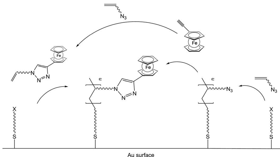
Scheme 4 One pot click reaction with competing pre- or post-synthetic ferrocene attachment to the polymer.
