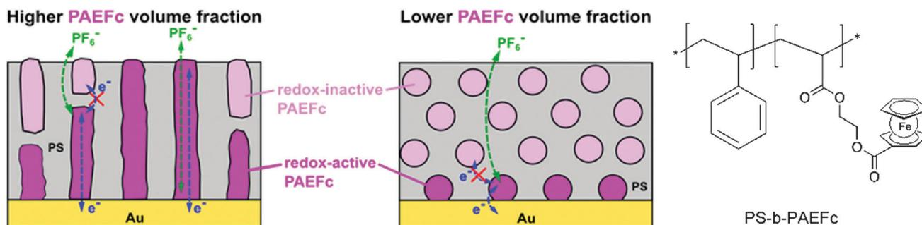
**Scheme 16** Microdomains of different sizes and shapes in thin films of ferrocene-containing diblock copolymers (left, reprinted with permission from ref. 11. Copyright (2015) American Chemical Society) and sketch of the polymer structure (right).
