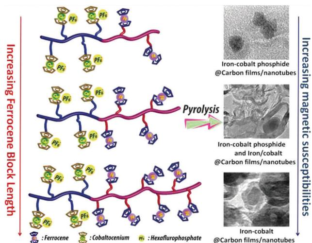
**Scheme 20** Variation of the metal ratio in heterobimetallic diblock copolymers and influence of the magnetic behavior. Reprinted with permission from ref. 42. Copyright (2014) American Chemical Society.
