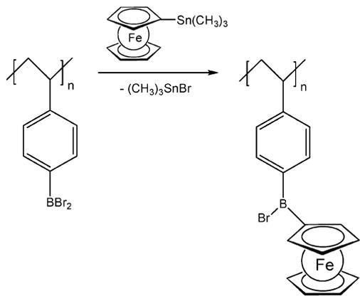
Scheme 8 Post-synthetic modification of borylated polystyrene with stannylferrocene.
